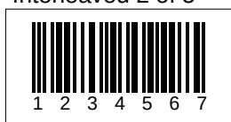
Interleaved 2 of 5 + CHECKSUM
